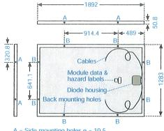
A = Side mounting holes Ø = 10.5 B = Back mounting holes Ø = 10.5 (all dimensions in mm)
